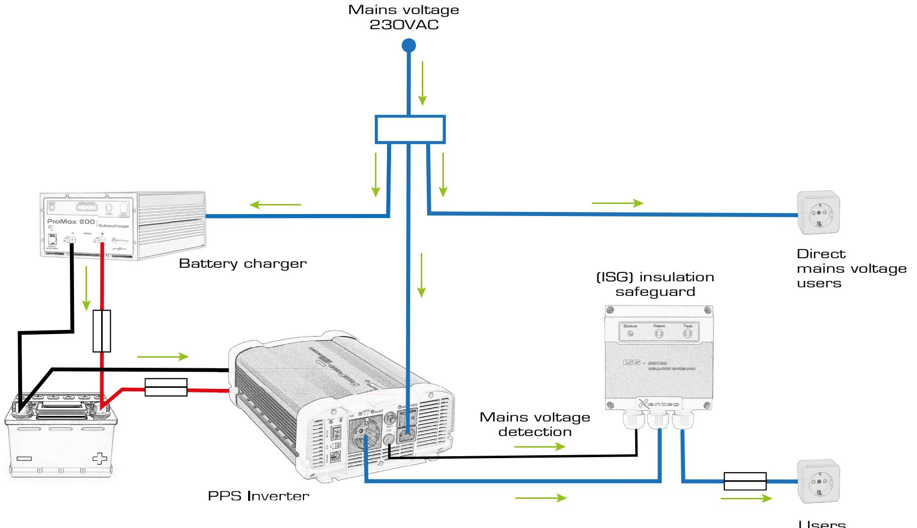
**Note:** Always connect the mains voltage detection (sense wire) connection of the insulation monitor to the 'MD' connector of the PurePowerSwitch. Use the cable that is supplied with the PurePowerSwitch. Never connect the mains voltage detection directly to the mains voltage!
